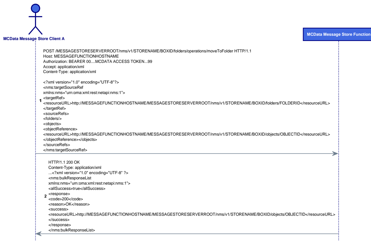
Figure 122mm: MCDATAMS/MOVE/01 Message Sequence
