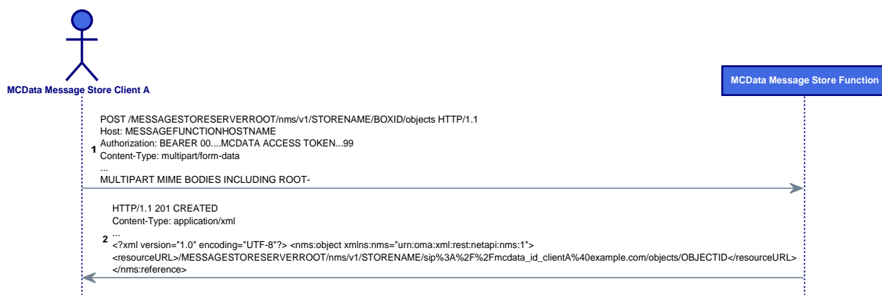
Figure 122mr: MCDATAMS/UP/01 Message Sequence
