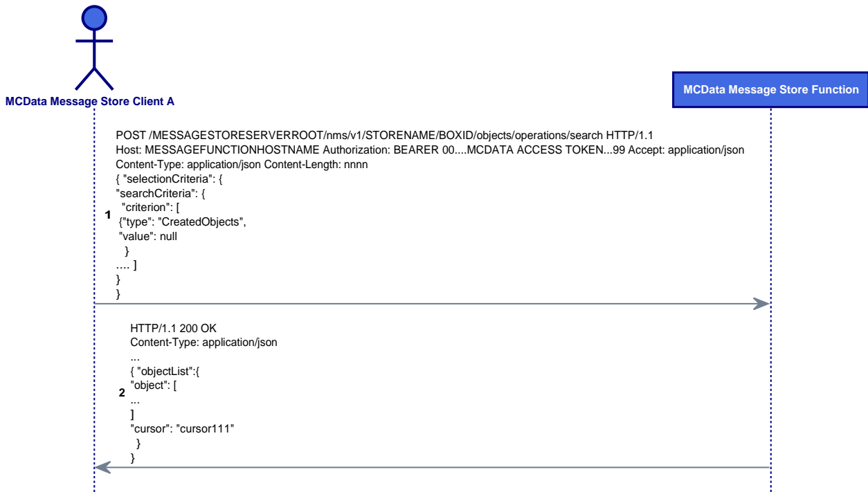
Figure 122mt: MCDATAMS/SYNC/02 Message Sequence
